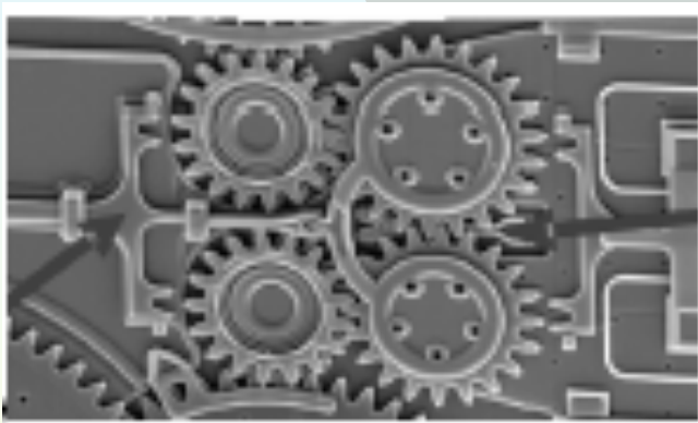
NanoEngrenages en polysilicium (diam des engrenages = 7\mu\text{m} )
