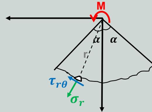
$$\begin{aligned}\sigma_r &= \frac{-2 M \sin 2\theta}{r^2 (\sin 2\alpha - 2\alpha \cos 2\alpha)} \\ \sigma_\theta &= 0 \\ \tau_{r\theta} &= \frac{M (\cos 2\theta - \cos 2\alpha)}{r^2 (\sin 2\alpha - 2\alpha \cos 2\alpha)}\end{aligned}$$
