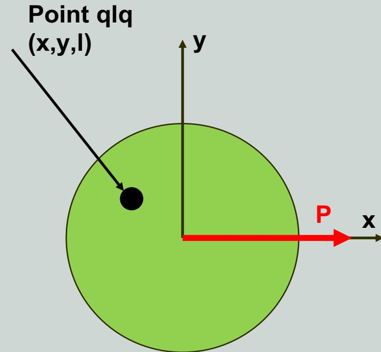
$$\begin{aligned} \sigma_x &= \sigma_y = \tau_{xy} = 0 \\ \tau_{xz} &= a \cdot x^2 + b \cdot y^2 + c \\ \tau_{yz} &= d \cdot x \cdot y \\ \sigma_z &= e \cdot x - 2(1 + \vartheta) \cdot (a + b) \cdot x \cdot z \end{aligned}$$
