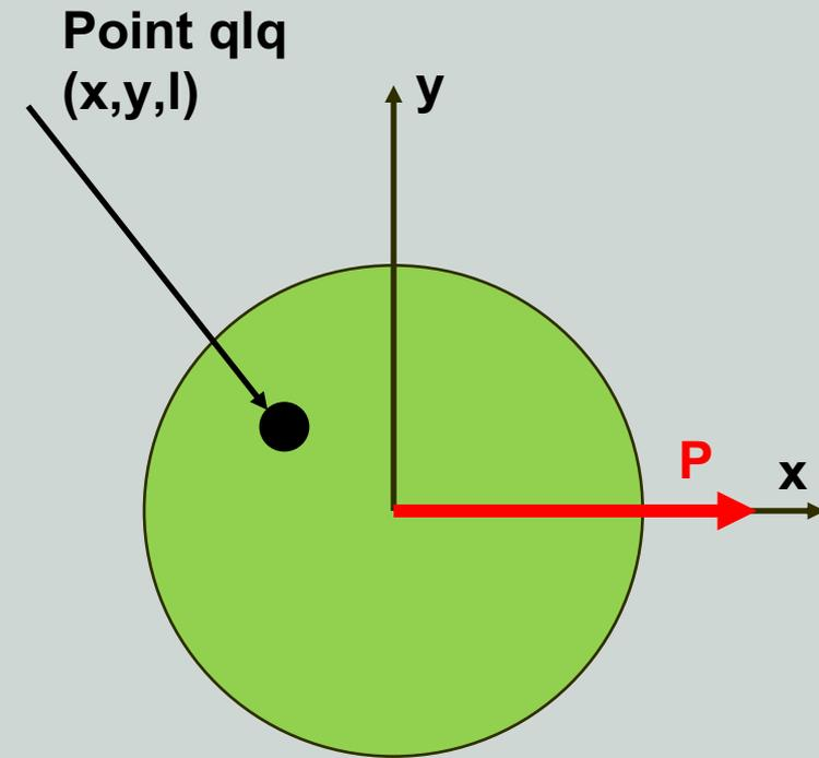
$$\begin{aligned}\sigma_x &= \sigma_y = \tau_{xy} = 0 \\ \tau_{xz} &= a \cdot x^2 + b \cdot y^2 + c \\ \tau_{yz} &= d \cdot x \cdot y \\ \sigma_z &= e \cdot x - 2(1 + \nu) \cdot (a + b) \cdot x \cdot z\end{aligned}$$
